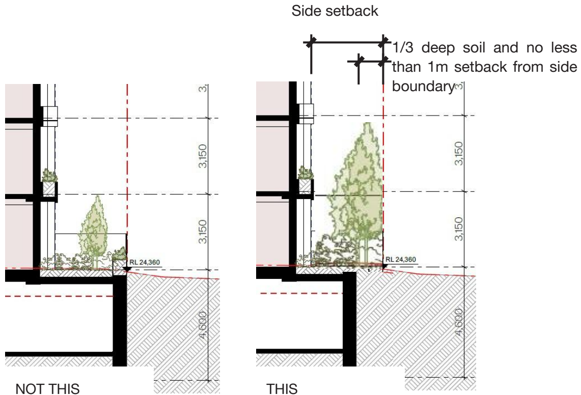
Figure 7: Screen planting in deep soil at the side boundary
