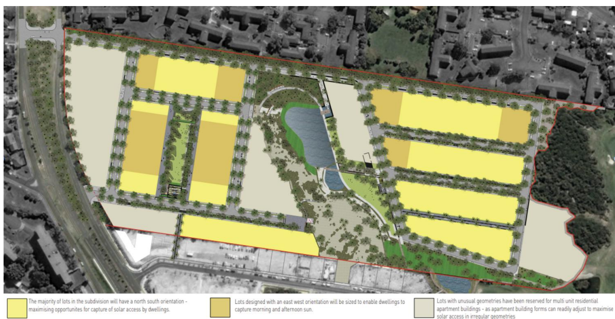
Figure 16: Solar orientation on the site
