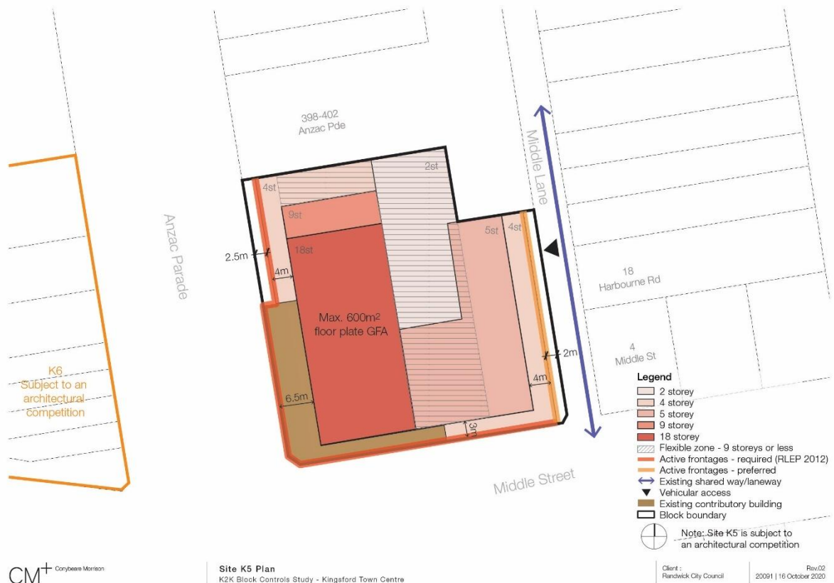
Figure 12: K5 Site block controls, Kingsford Midtown
