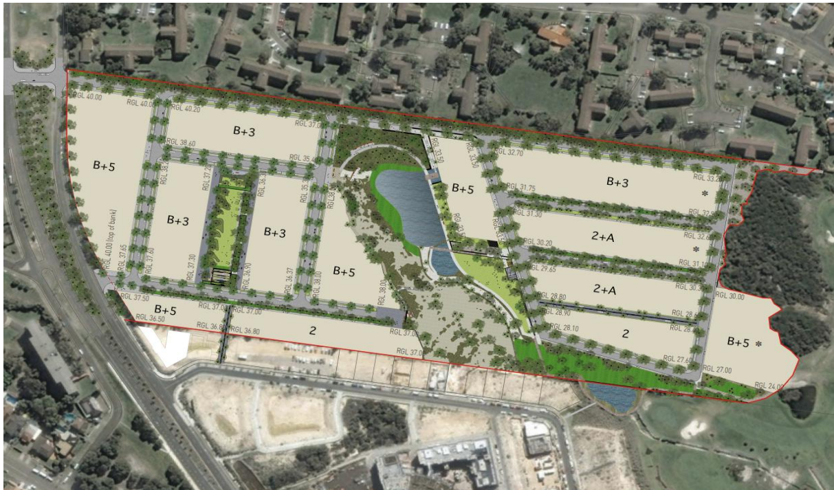
Figure 22: Building height control plan
