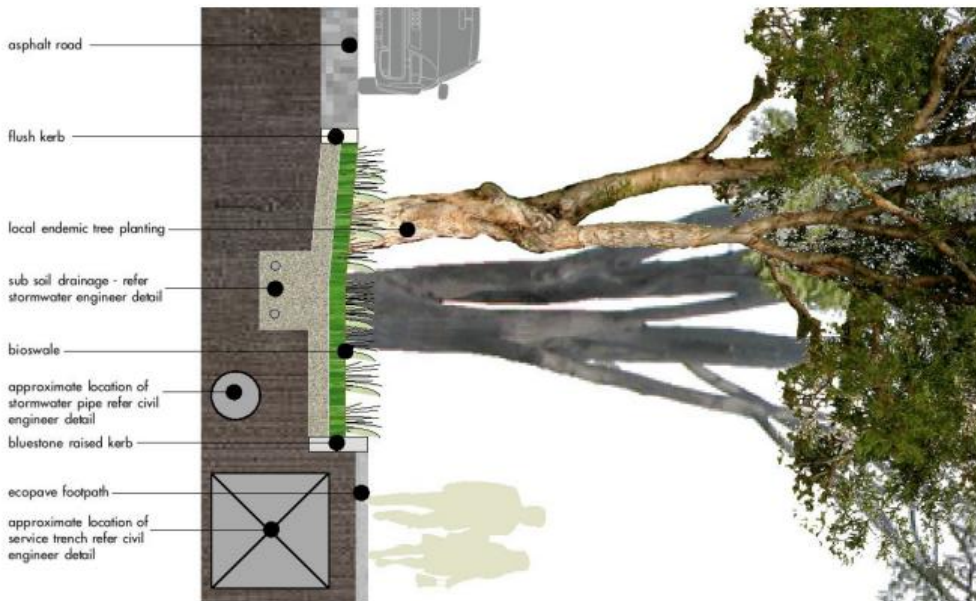
Bioretention swale - Raingarden streets
