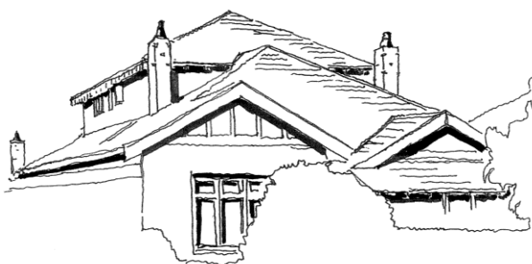
Figure 10: Additions set back from the existing ridgeline retain the form and detail of the existing residences. Use of simple roof forms and subtle detailing further enhances the relationship of new and existing works.
