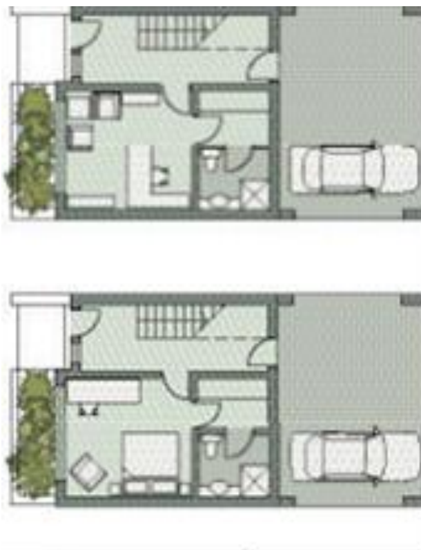
Figure 68: The layout on the ground floor of this 2-storey apartment facilitates a variety of uses: small business, third bedroom, shared housing for independent adults and housing for an elderly parent
